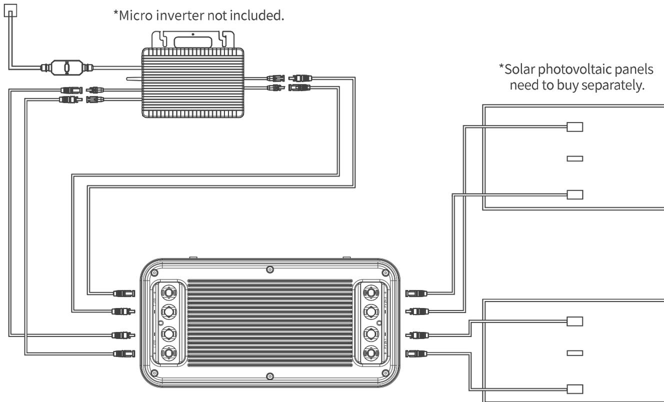
If you find that the micro inverter is not functioning properly after the connection described above, please connect as follows: Connect one of the micro inverter to the Output1 of the product, and the other micro inverter should either be disconnected or connected to the solar energy.
