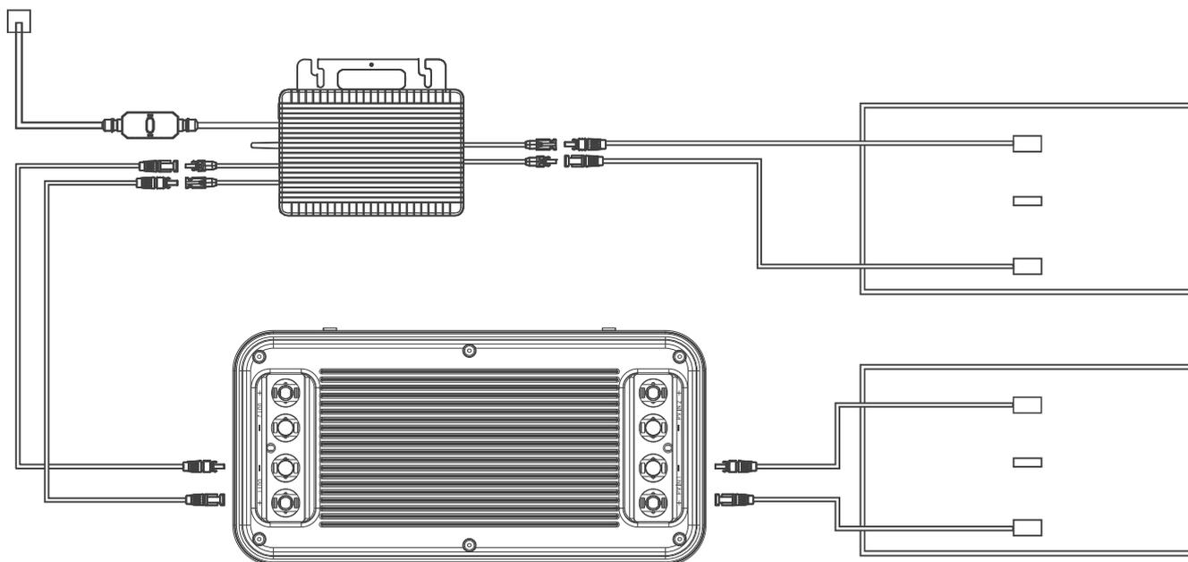
\*This issue arises from the fact that some of the micro inverters available on the market have a common internal reference point. When both micro inverters are connected to a battery bank simultaneously, the micro inverter will function abnormally.
