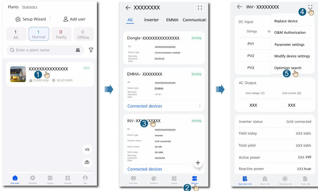
**Step 7** Choose **Devices > Connected devices > Optimizer**, tap **Optimizer No.**, select the faulty optimizer, tap **Device Replacement**, and replace the optimizer as prompted.
