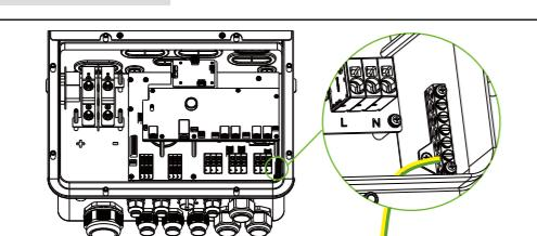
The Ground cable should be connected to the ground terminal on the grid side to prevent electric shock.
