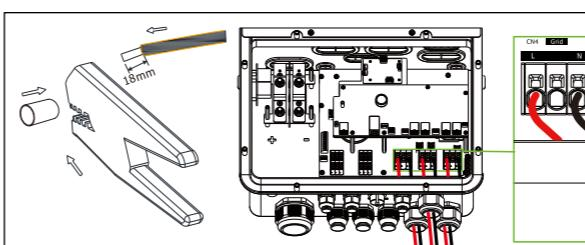
The AC circuit breaker must be turned off before connecting the grid, load and generator ports.
