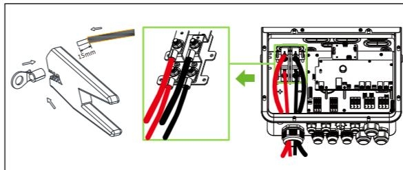
1. Strip 0.59 inches (15 mm) of the battery cable insulation.
