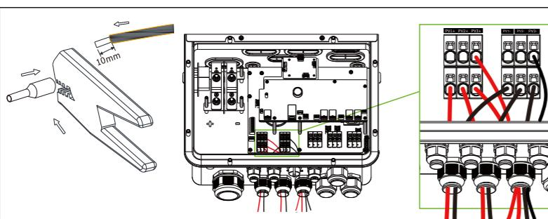
1. Strip 0.39 inches(10 mm) of PV cable insulation.
